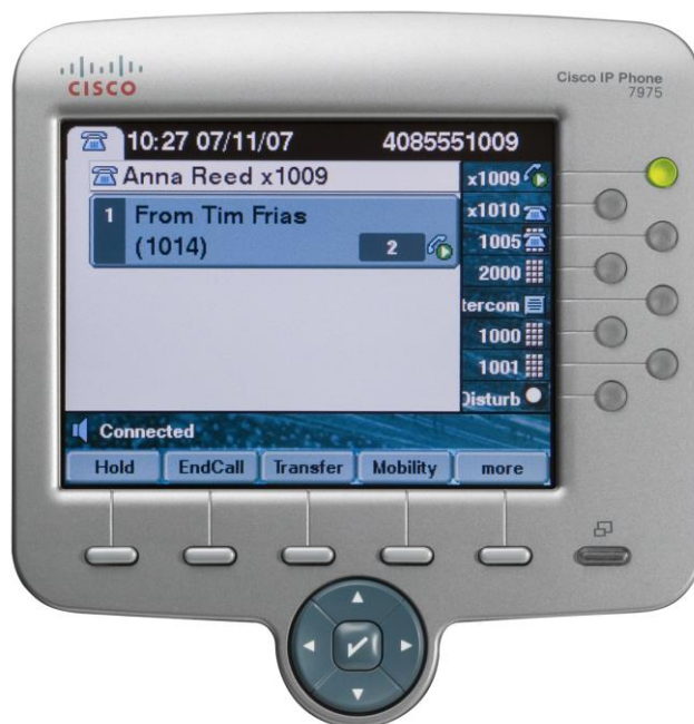
Figure 2. Close-Up of Display and Lighted Line Keys
